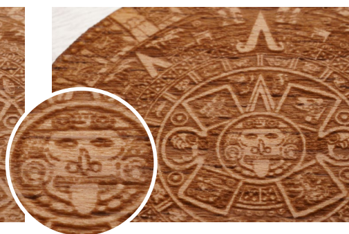
4.0" engraving A rough engraving that looks blurred
